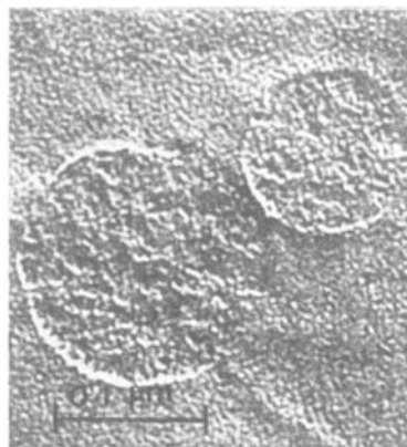
FIG. 2. The appearance of the internal structure of polymethylcyanoacrylate nanocapsules by the electron microscopy after spray freezing and cryofracture (see (Bachmann et al 1973) for details).
